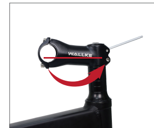
1. Release side stem bolts Rotate 180 degree
