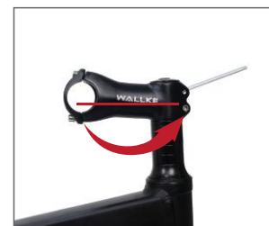
1. Release side stem bolts Rotate 180 degree
